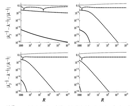
**Figure 2.** Relative errors of  $\lambda^{-1/2}$ , computed via the iterations of (18) and the Haaland formula (eq 4), as functions of the Reynolds number *R*. (upper-left) K = 0. (upper-right)  $K = 10^{-3}$ . (lower-left)  $K = 10^{-2}$ . (lower-right)  $K = 10^{-1}$ : (dotted line)  $\lambda_0^{-1/2}$ ; (dashed line)  $\lambda_1^{-1/2}$ ; (solid line)  $\lambda_2^{-1/2}$ ; (dashed-dotted line)  $\lambda_{\rm H}^{-1/2}$  (Haaland's approximation).
